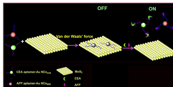
Scheme 1. Schematic illustration of the dual color FRET biosensor for simultaneous detection of multiple tumor markers.
