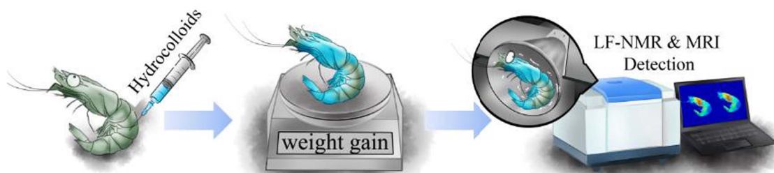
Fig. 1. Schematic illustration of a typical LF-NMR and MRI experimental workflow for the detection of prawns injected with hydrocolloids.
