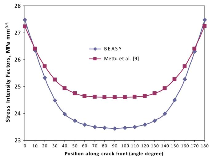
Fig. 2. Comparison of the SIF values for longitudinal semi-elliptical crack on inner surface of tube obtained by using BEASY [7] and by Mettu et al. [9] ( $a/c = 1$ ;  $a = 0.5$  mm).
