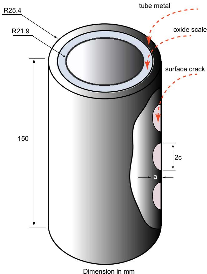
Fig. 1. Studied model of the multiple surface cracks on the outer surface of a water-tube boiler in the presence of the oxide scale.
