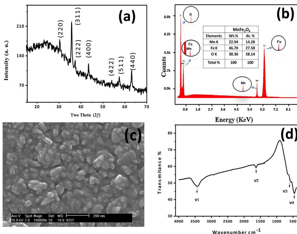
Fig. 1. (a) XRD ( $2\theta$  as deg.), (b) EDAX, (c) FESEM, (d) FT-IR measurements of  $\text{MnFe}_2\text{O}_4$  film deposited on glass substrate.
