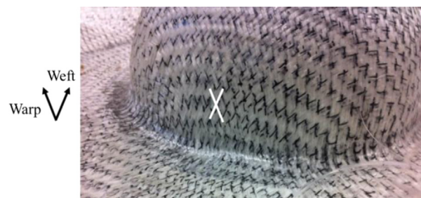
Fig. 1. Deformation of textiles due to forming processes (a) fiber reorientations and (b) manufacturing defects.
