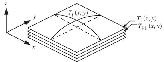
Fig. 3. Schematic of the temperature field in layer *i*.
