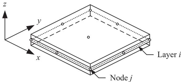
Fig. 2. Shell heat transfer element.
