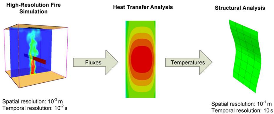
Fig. 1. Transfer of thermal data across disparate scales in modeling structures in fire.
