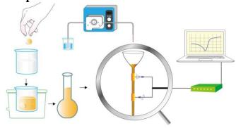
By employing an electrical micro-titration system, in which a capacitively coupled contactless conductivity detector is used to monitor the reaction process in real time, ciprofloxacin hydrochloride in tablet samples is determined. Because the reaction solutions are isolated from the working electrodes, it shows significant simplicity and cost-effectiveness, by eliminating the requirements for detector exchange/renewal between measurements, and by involving no auxiliary chemicals.
