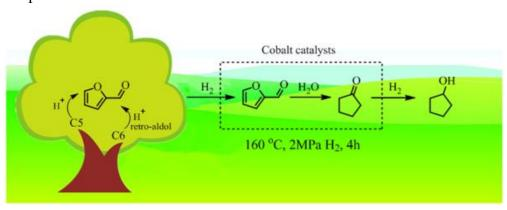
A series of cobalt catalysts with different supports were prepared for the selective conversion of biomass-derived furfural to cyclopentanol in one step. The best CPL yield was 82 mol% at 160  $^{\circ}$ C, 2 MPa H<sub>2</sub>, 4 h when cobalt was supported on tetragonal zirconia that can be obtained by doping La<sub>2</sub>O<sub>3</sub>.
