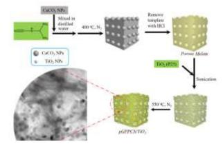
Porous graphite-phase polymeric carbon nitride (GPPCN)/TiO<sub>2</sub> donor-acceptor heterojunction was facilely fabricated through the combination of a template technique with a co-calcination process, which exhibited much higher photoelectric activity compared to pristine carbon nitride and TiO<sub>2</sub>.
