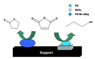
The types of alloy phase and the amounts of the surface Pd-SnO(x) sites altered along with Sn/Pd mass ratios from 0--1.0 synthesized in the process of preparation. The maximum reaction rate was 0.57 mol-GBL/(mol-Pd-min) and selectivity was 95.94% when the Sn/Pd mass ratio was 0.6. It might be attributed to the formation of  $Pd_2Sn$  alloy and less amounts of Pd-SnO(x) sites.
