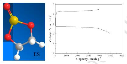
An ethylene sulfite based electrolyte was used in non-aqueous lithium-oxygen batteries, and the batteries showed high specific capacity, good round-trip efficiency and cycling stability.
