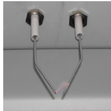
Fig. 6 – Ignition source mounted in the roof of the container.
