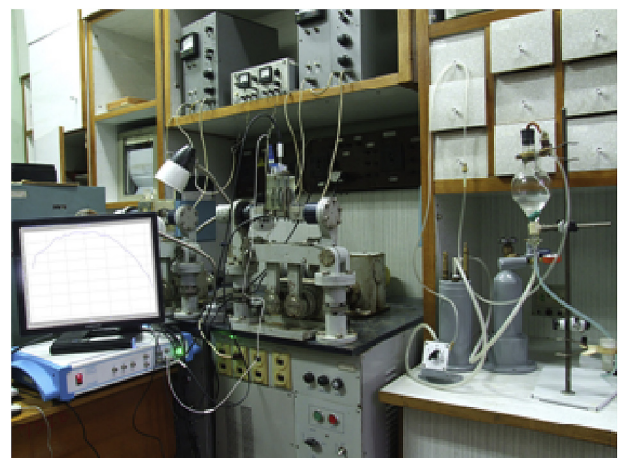
Fig. 3 – Special fatigue testing stand.
