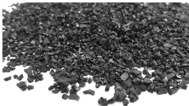
Fig. 1 – Granular activated carbon with particle size of 2–3 mm as microbial support carrier.
