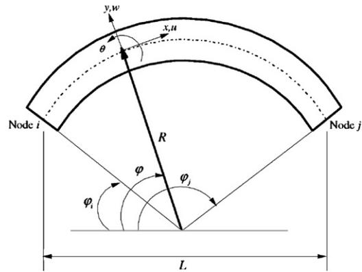
Fig. 1. Description of the curved beam element.
