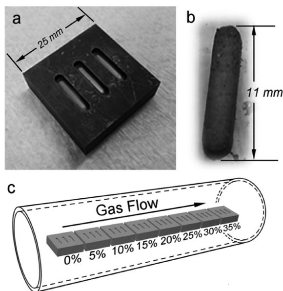
**Fig. 1.** (a) Graphite mold used in processing the samples. (b) Typical sample pellet after release from the mold. (c) Arrangement of the samples in the tube furnace for heat treatment.
