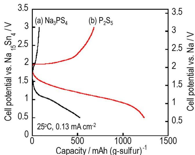
Fig. 1. The 1st discharge-charge curves of the all-solid-state Na/S cells with a sulfur composite electrode of S-KB-Na<sub>3</sub>PS<sub>4</sub> (a) or S-KB-P<sub>2</sub>S<sub>5</sub> (b) at 25 °C at a current density of 0.13 mA cm<sup>-2</sup>.
