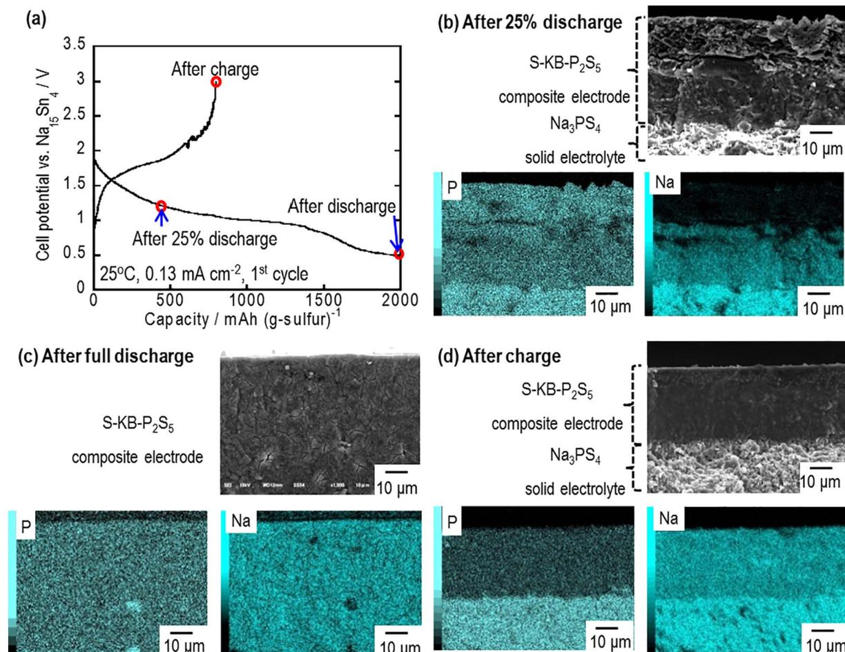
Fig. 2. (a) The 1st discharge-charge curves of the all-solid-state Na/S cells with a sulfur composite electrode of S-KB-P<sub>2</sub>S<sub>5</sub> with a S:KB:P<sub>2</sub>S<sub>5</sub> weight ratio of 45:19:36 at 25 °C at a current density of 0.13 mA cm<sup>-2</sup>. SEM and EDX mapping images of a cross-section of the S-KB-Na<sub>3</sub>PS<sub>4</sub> composite electrode after 25% (b) and full (c) discharge and charge (d) processes.
