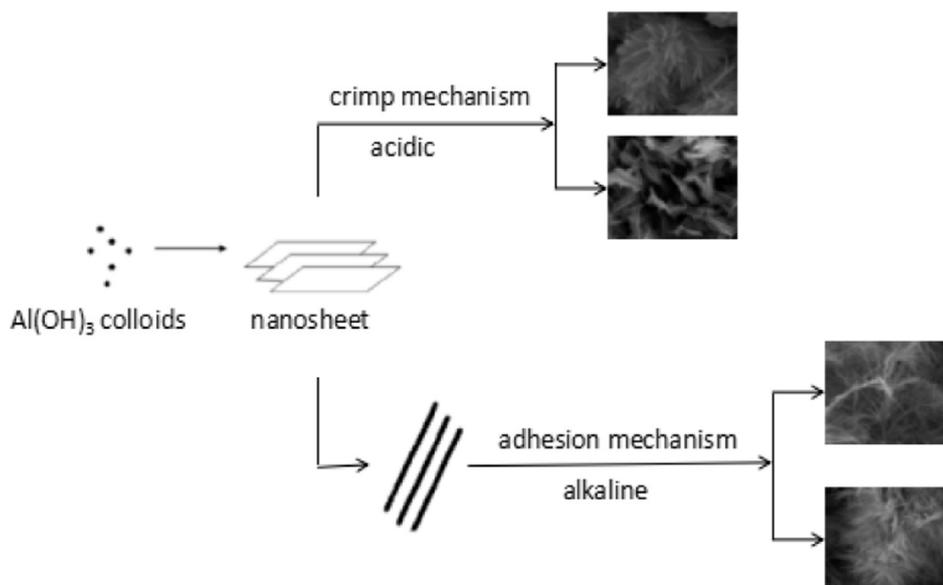
**Fig. 2.** Schematic illustration for the growth process of the precursor aluminum.
