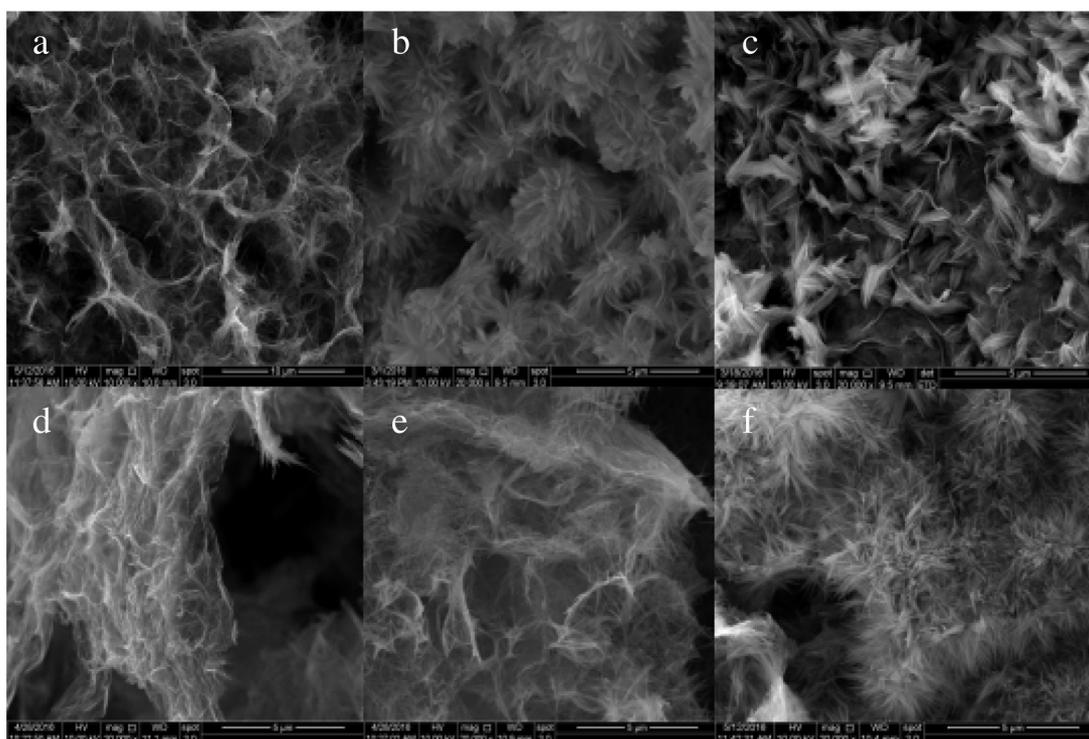
**Fig. 1.** SEM images of a typical as-synthesized sample at different pH. (a) pH = 2 (b) pH = 4 (c) pH = 6 (d) pH = 8 (e) pH = 9 (f) pH = 10.
