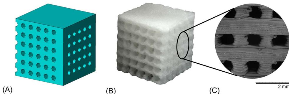
Fig. 1. 3D model of a scaffold (A), 3D-printed PLA/HA scaffold (B) and SEM image of its structure (C).
