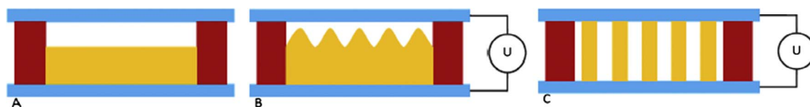
Fig. 1. (Blue: electrode; red: spacer; yellow: patternable fluid.) (A) no applied voltage. (B) initial instability. (C) fully-evolved structure. (For interpretation of the references to colour in this figure legend, the reader is referred to the web version of this article.)
