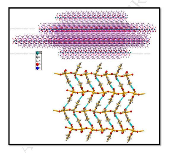
Polymeric layer 1-D (Top) and Helical type 2-D (bottom) bonding fashion of complex 1 viewed along the b axis.
