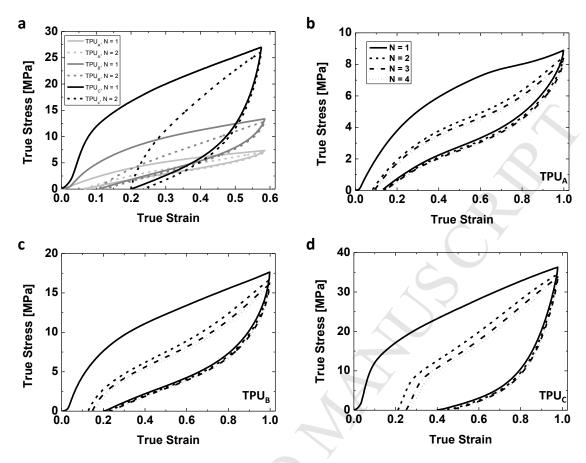
Large strain behavior of thermoplastic polyurethanes spanning a range of fractions of hard and soft segment contents: shape recovery and energy dissipation upon cyclic loading conditions are highly dependent on the fractions of hard and soft contents, travelling between those in glassy and rubbery polymers.
