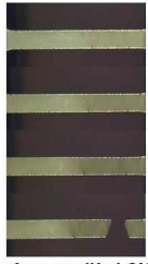
Surface modified CNC induced shear bands
