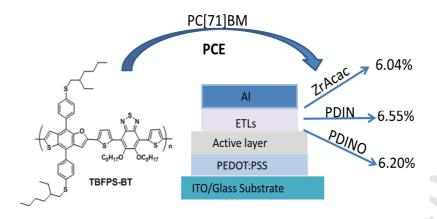
With a new alkylthio phenyl substituted TBF polymer and PC[71]BM as the active layer, the best PCE for device of 6.55% was obtained with PDIN as ETL.
