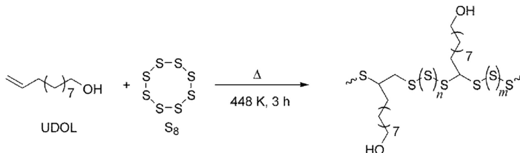
Scheme 1. Preparation route of poly(S- r -UDOL) from sulfur (S) and 10-undecen-1-ol (UDOL), n and m > 0–8.
