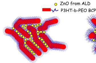
Poor PEO solvent Collapsed PEO Limited ZnO incorporation
