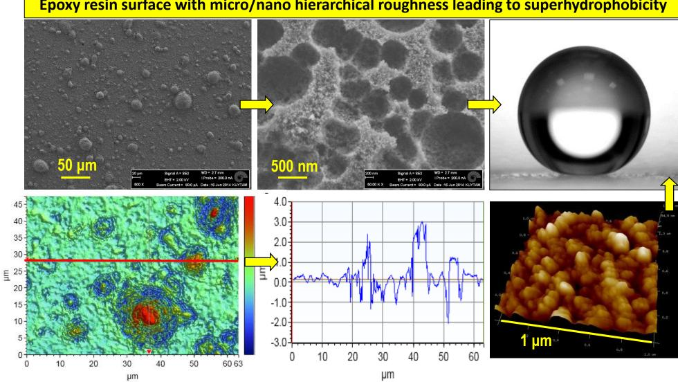
Epoxy resin surface with micro/nano hierarchical roughness leading to superhydrophobicity
