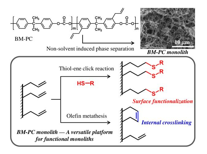
A polycarbonate monolith that carries allyl side groups was fabricated by a simple phase separation technique. With the porous network structure largely maintained, the monolith could be modified by using the thiol-ene click chemistry and olefin metathesis, which qualifies the present monolith as a versatile platform for a wide range of functional monoliths.
