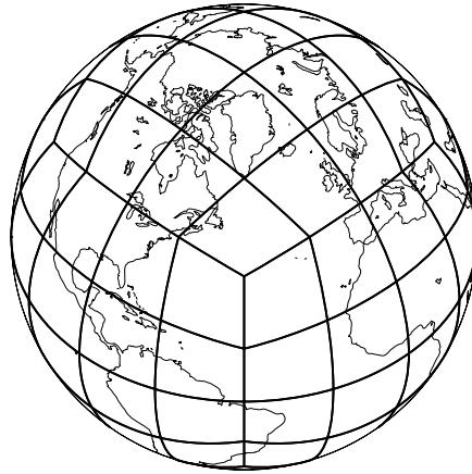
Fig. 1. Tiling the surface of the sphere with quadrilaterals. An inscribed cube is projected to the surface of the sphere. The faces of the cubed-sphere are further subdivided to form a quadrilateral grid of the desired resolution. The gnomonic equal angle projection is used, resulting in a quasi-uniform but non-orthogonal grid [44].
