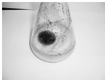
Fig. 1. Picture of a precipitation polymerization process at 50% monomer conversion showing that all the CNTs are entrapped in the precipitated polymer.
