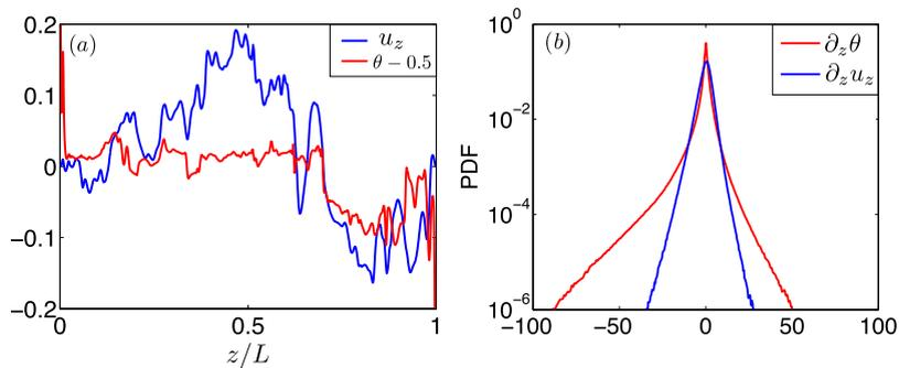
**Fig. 2.** (a) Instantaneous  $\theta$  and  $u_z$  profiles as a function of the vertical coordinate  $z/L$  for  $Ra = 10^{10}$ ,  $Pr = 1$  RB simulation. (b) PDF of  $\partial_z \theta$  and  $\partial_z u_z$  for the same simulation in the bulk.
