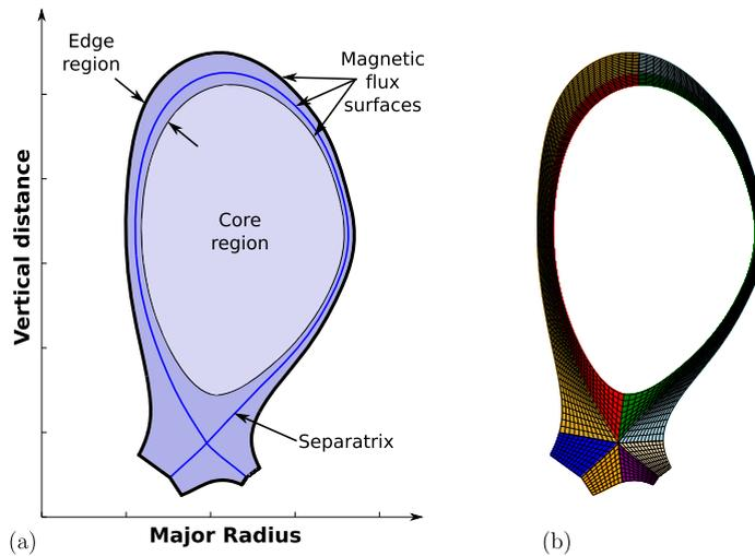
**Fig. 1.** Poloidal cross section of the single-null magnetic field geometry in a tokamak fusion reactor showing (a) the edge and core regions and the separatrix that separates open and closed magnetic field lines and (b) the decomposition of the single-null domain into eight blocks.
