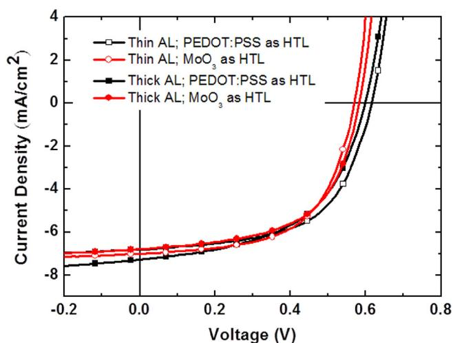
Fig. 2. Current-voltage curves of four types of spin-coated devices based on two active layer thicknesses and two HTLs (PEDOT:PSS and  $\text{MoO}_3$ ).
