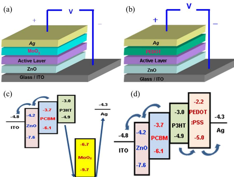
Fig. 1. The schematics of devices and the corresponding bandgap diagram based on (a, c)  $\text{MoO}_3$  and (b, d) PEDOT:PSS as the HTL.
