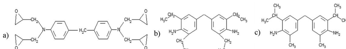
**Fig. 1.** Chemical structure of a) the epoxy resin tetraglycidyl methylene dianiline and the hardeners, b) the 4,4'-methylenebis(2-isopropyl-6-methylaniline) and c) the 4,4'-methylenebis(2,6-diethylaniline).
