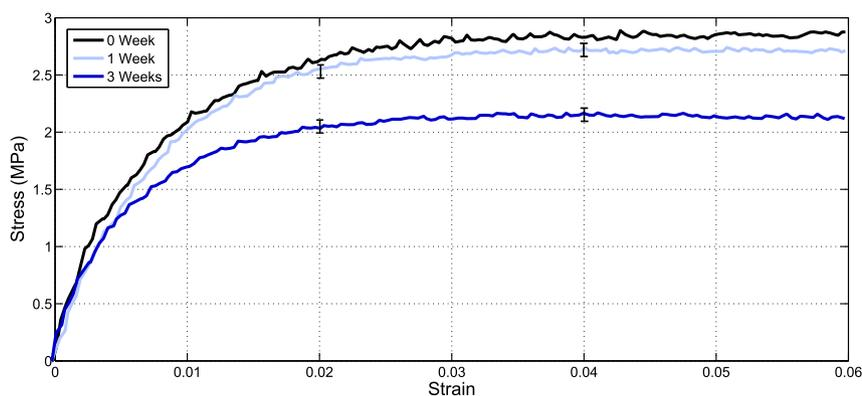
Fig. 1. Experimental load curves at 6% strain load at 0, 1, and 3 weeks of degradation.
