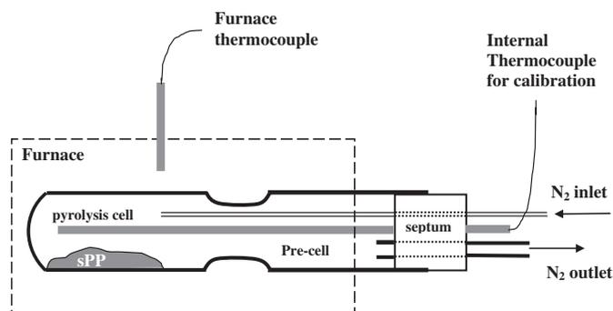
Fig. 1. Scheme of the pyrolysis set-up.
