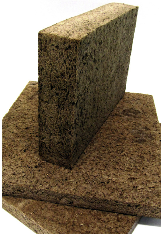
Fig. 1. Rigid insulating panels from flax short fibres and protein binder.
