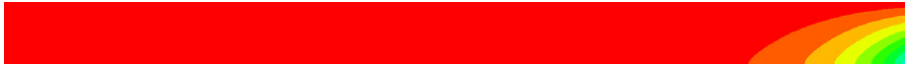
Fig. 1. Non-dimensional pressure field for a laminar boundary layer developing over a flat plate obtained with the classical outlet condition.
