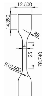
Fig. 2. Dumbbell specimen final used for the crack nucleation experiments. Dimensions satisfy the BS ISO 6943:2011 standard [31].
