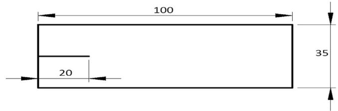
Fig. 1. Rectangular specimens used for the crack growth experiments. All dimensions are in mm.
