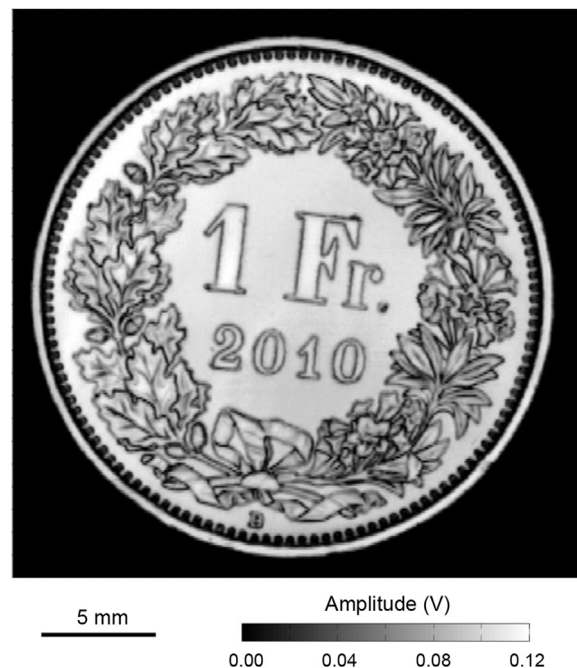
Fig. 2. Amplitude C-scan of the surface of a 1 Swiss Franc coin.
