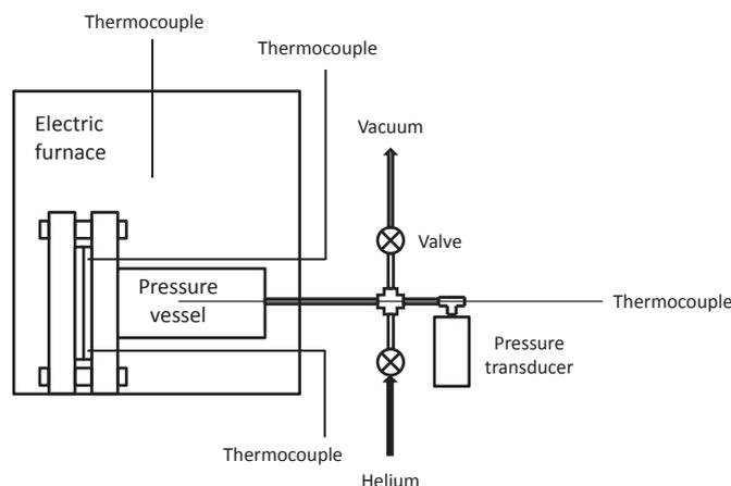
Fig. 1. A schematic illustration of the experimental apparatus.
