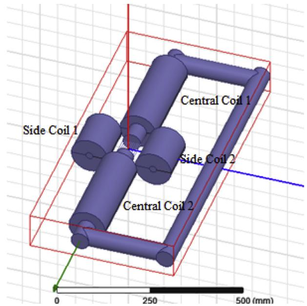
Fig. 2. 3D schematic showing position of electromagnets.
