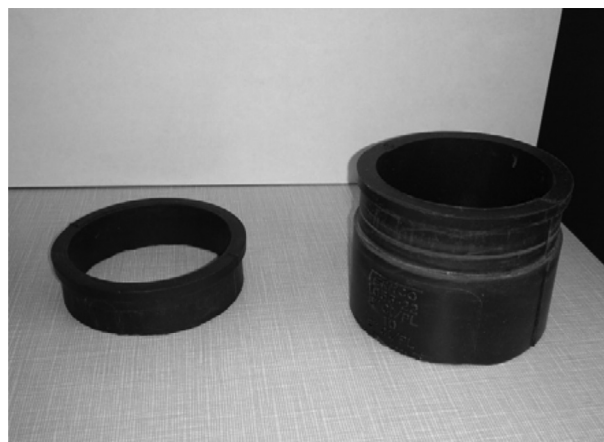
Fig. 2. (Left) PVC flexible rubber coupler was cut to be 1.0 in. tall for the top of the dome (Right) PVC flexible rubber coupler was cut to be 3.0 in. tall for the bottom of the dome.
