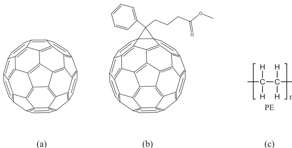
Fig. 1. Chemical structures of: (a)  $\text{C}_{60}$ ; (b) PCBM and (c) Polyethylene (PE).
