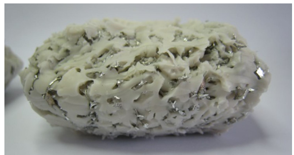
Fig. 2. De-bonding of silicone filler from compressed metal foam.
