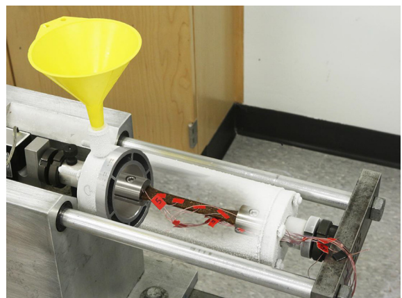
Fig. 3. Cold chamber cutaway, showing coolant passages, round grips and thermocouples.
