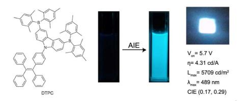
A novel compound based on tetraphenylethene, carbazole and dimesitylboron moieties with aggregation induced emission (AIE) properties was synthesized and utilized as a highly efficient blue light-emitting material in OLEDs.
