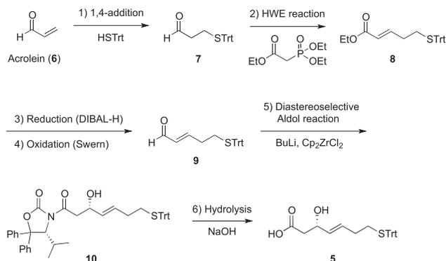
Fig. 2. Current synthesis of (*E*)-(*S*)-3-hydroxy-7-tritylthio-heptenoic acid (**5**).
