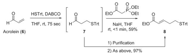
Scheme 1. Initial attempt of the one-pot synthesis of **8** in a batch system.
