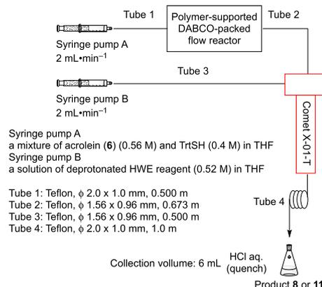
Fig. 3. Flow system for the synthesis of  $\alpha, \beta$ -unsaturated esters **8** and **11**.
