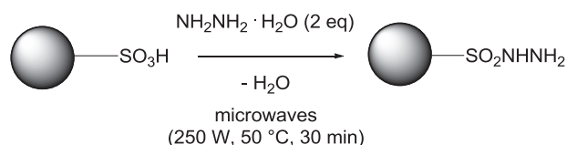
Fig. 4. Microwave synthesis of polymer-bound sulfonylhydrazide.
