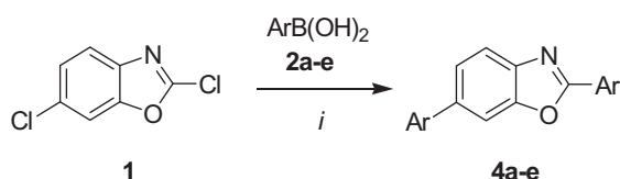
Scheme 4. Synthesis of 4a–e . Reagents and conditions: i, 1 (1.0 equiv), 2a–e (2.2 equiv), Pd(PPh 3 ) 4 (26 mg, 6 mol %), K 2 CO 3 (aqueous solution, 2 M), 1,4-dioxane, 120 °C, 8 h.
